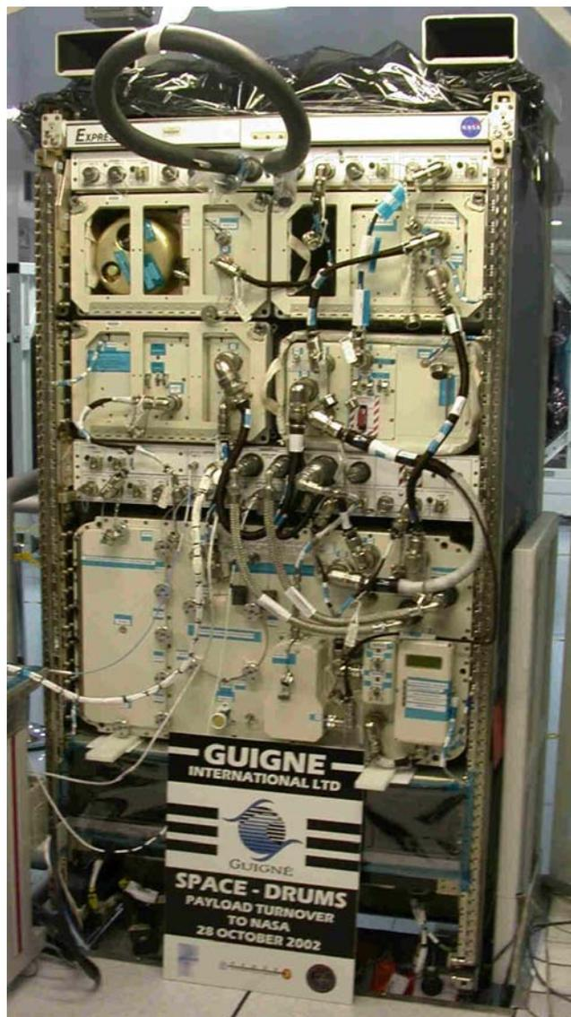
**Figure 3 - Space-DRUMS payload mounted in an EXPRESS rack for online testing at Kennedy Space Center.**
