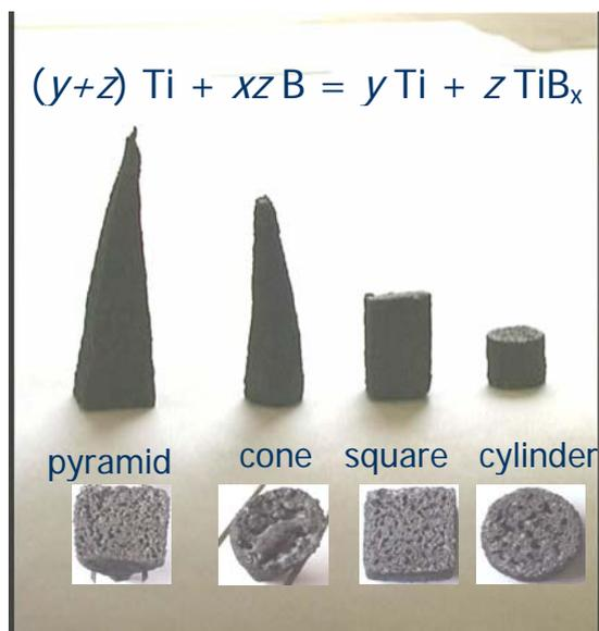
**Figure 1 - near net shape processing of a ceramic-metal composite using SHS.**
